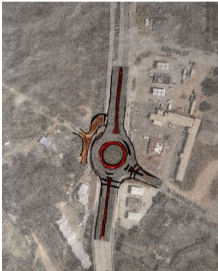
Figure 35: Potential Three-leg Roundabout
